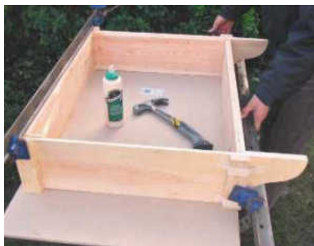
STEP 9. Dry assemble the carcass to check everything fits correctly, then glue up with sash cramps, checking for square
